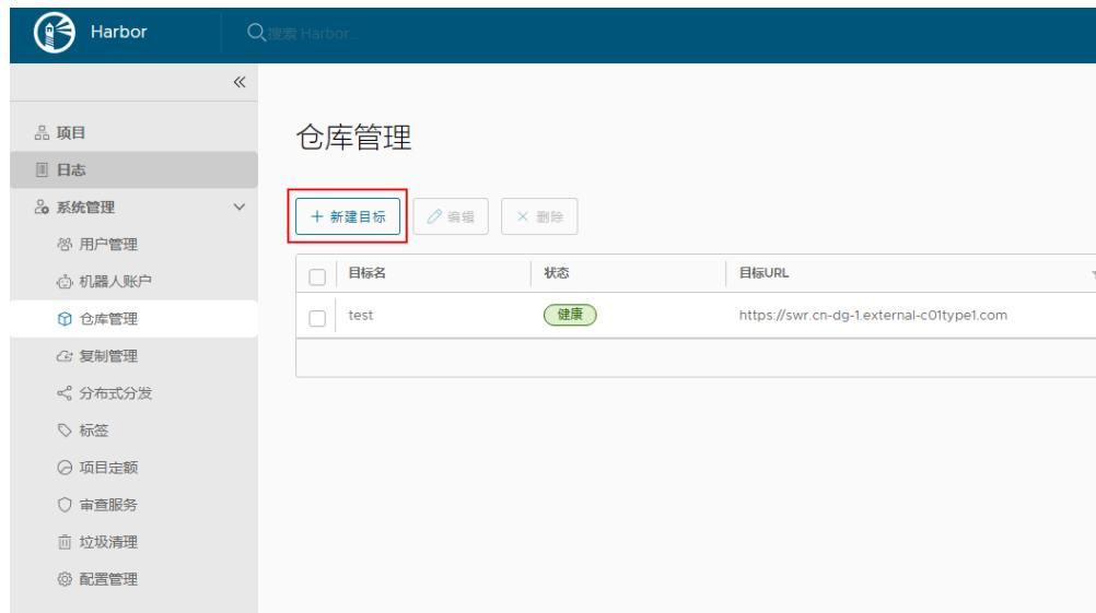
The screenshot shows the Harbor interface with the sidebar navigation expanded. Under '仓库管理' (Warehouse Management), the '目标' (Target) option is selected. A red box highlights the '+ 新建目标' (New Target) button. Below it, there is a table listing one target named 'test' with a green '健康' (Healthy) status and the URL 'https://swr.cn-dg-1.external-c01type1.com'.
